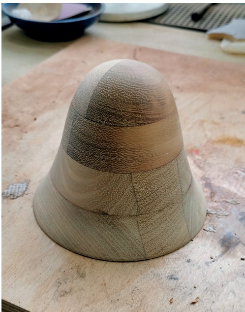
Bell shape comprising four layers of multiple Iroko straps
